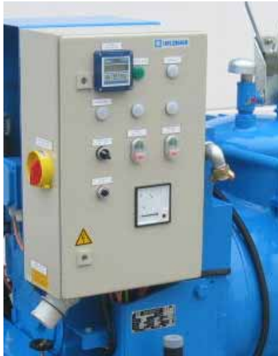
Electrical control kit and potentiometer for mixing time setting
