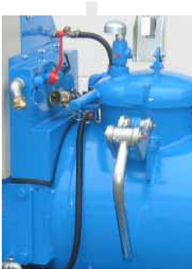
Air armature with upper and lower air controls. Lid with safety valves
