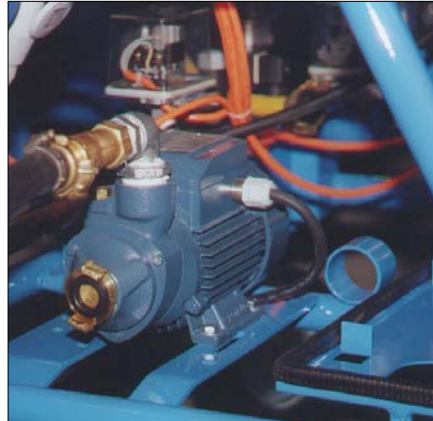
Housing for water booster pump. It can be mounted onto the machine frame
