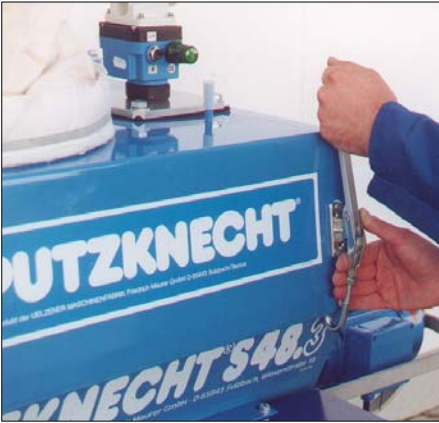
Easy assembly of feeding hood thanks to lever locking hooks and special profile edges
