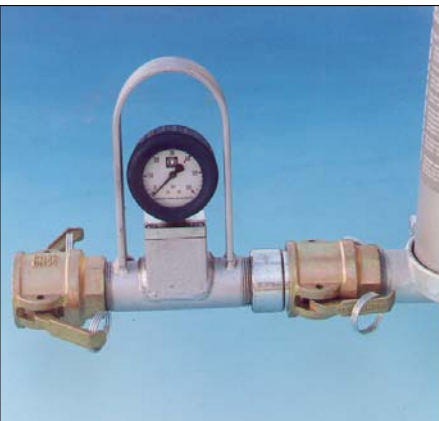
The pump outlet with standard coupling SKM35 is equipped with detachable mortar pressure gauge as required by the trade association due to safety regulations.
