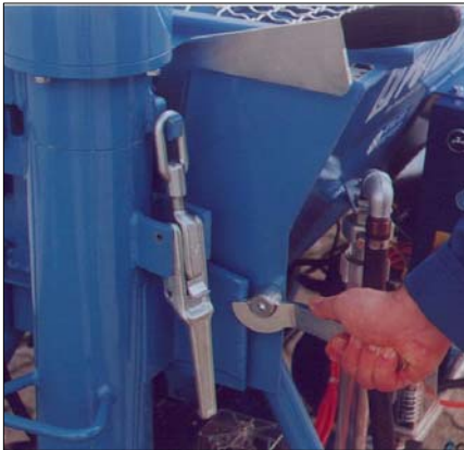
Handy locking system for a tight positioning of the mixing chamber
