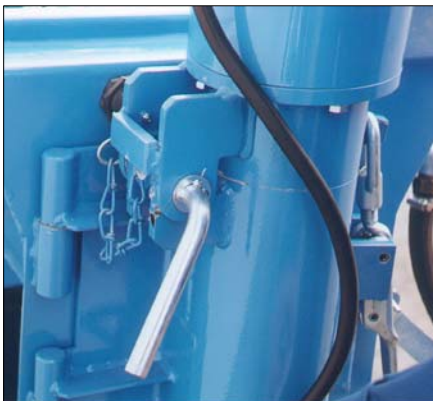
Detachable pump motor for easy transport without tools.
