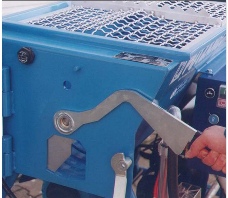
Improved separator between dry hopper and mixing chamber. Work can be stopped also with a full load of dry material.
