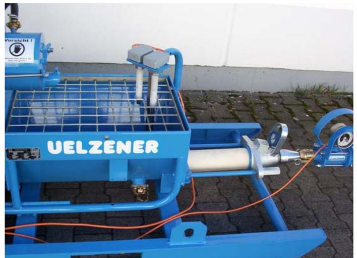
The injection unit might be equipped with a mortar pressure control (Part no. 130.09.101.1), which will switch off the mortar pump when reaching the adjustable conveying pressure.
