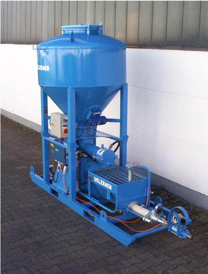
The compact injection unit E407KM-K-C mounted on a skid frame is used for back filling of concrete tubing segments, well sinking, geothermal energy units; water piping, injection of rock anchors, injection of prestressing elements and many other applications, which do require a homogenous solubilized binder dispersion or pastry consistence.
